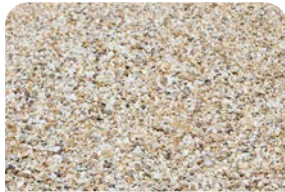
Exposed Aggregate Concrete
