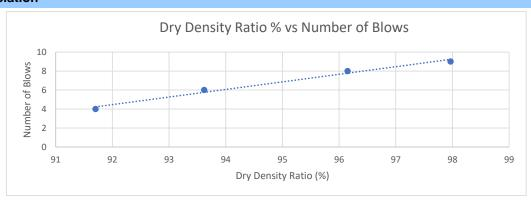
The results indicate that 7 blows are required to obtain a Dry Density Ratio of 95 %
